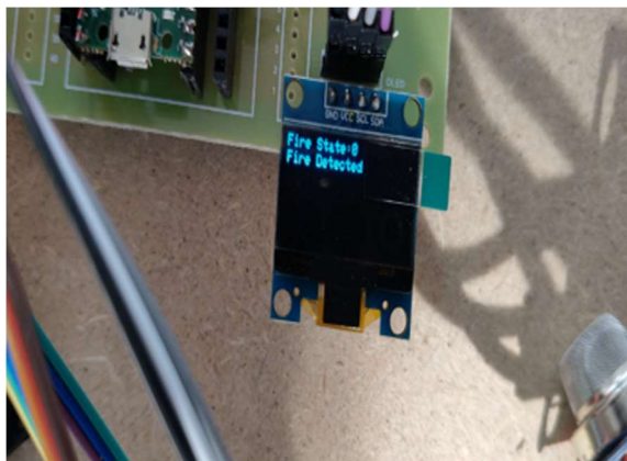
Fig 7: Oled Displaying Fire Is Detected
