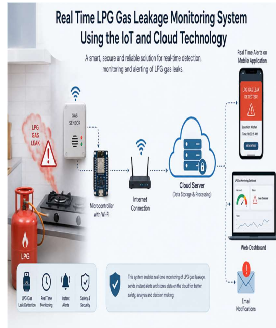
Figure 1: LPG Gas Leakage Monitoring System
